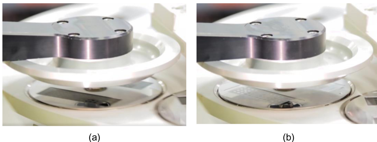
FIG. 4. Picture of the sputter coating process established at Stratec Consumables for high volume throughput. (a) Two black carbon PP substrates are automatically loaded into the sputter coating machine and (b) unloaded after the sputter coating process of the metal film. The metal coating is done homogeneously across the whole substrate surface.
